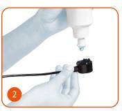
Apply the gel on the ultrasound transducer.
