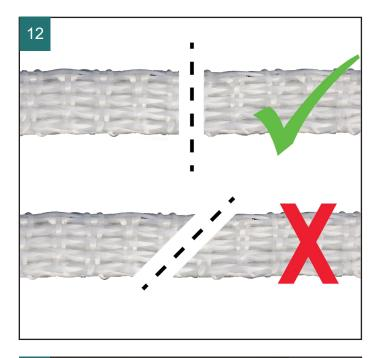
NOTE: Cut the Tube-Tape at right angles to its length to minimize the generation of loose fibres. Take care to remove any loose fibres that are created.
