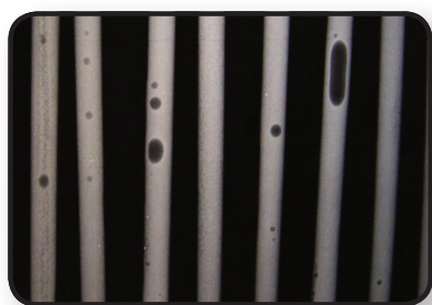
Bone cement mixed with a vacuum mixing system without collection under vacuum. High occurrence of macropores. 32
