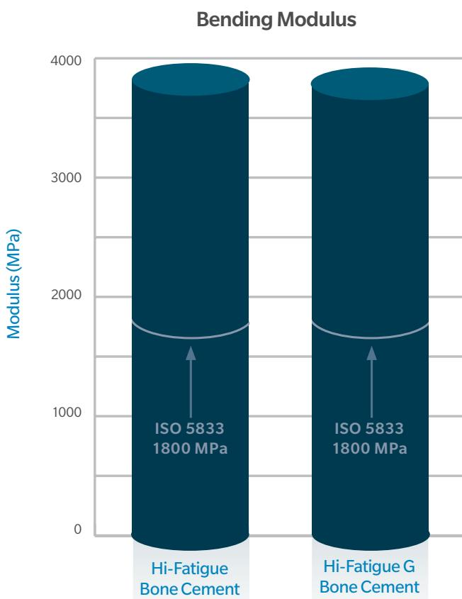
The minimum standard for bending strength of 50 MPa and the minimum standard for bending modulus of 1800 MPa as specified by ISO 5833 were fulfilled and exceeded by both the Hi-Fatigue Bone Cement and the Hi-Fatigue G Bone Cement.<sup>2\*</sup>
