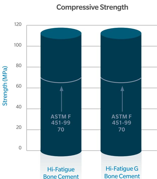
The minimum standard for compressive strength of 70 MPa, as specified by ASTM F451-16 and ISO 5833, were fulfilled and exceeded by both the Hi-Fatigue Bone Cement and the Hi-Fatigue G Bone Cement.<sup>2\*</sup>
